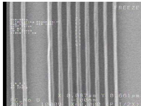
Figure 10. Top-down SEM image of 100 nm 1:1 lines and spaces for a TFE containing copolymer imaged at 157 nm using an alternating phase shift mask. The resist thickness is 164 nm.
