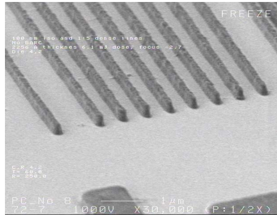
Figure 11. Tilt SEM image of 100 nm isolated and 1:5 lines and spaces in a 226 nm thick film of a vinyl addition copolymer of functionalized norbornenes exposed at 157 nm. The lines are oversized.
